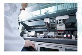
This 10 m3 mini-lab combines a comprehensive repertoire of basic laboratory equipment and high-end fluorescence micropolate readers operated by multifunctional pipetting and gripper arms. Barcode-controlled sample management is implemented by an integrated carousel and incubator. The lab on the second floor of the ZBSA had to be completely rebuilt and adapted to the needs of this robotic platform.
