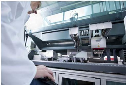
This 10 m3 mini-lab combines a comprehensive repertoire of basic laboratory equipment and high-end fluorescence micropolates readers operated by multifunctional pipetting and gripper arms. Barcode-controlled sample management is implemented by an integrated carousel and incubator. The lab on the second floor of the ZBSA had to be completely rebuilt and adapted to the needs of this robotic platform.
